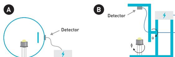
Typical measurement equipment for optical performance of LEDs—an integrating sphere (A) or a goniometer (B).
