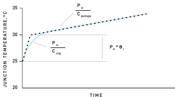
A simple model for the rise in junction temperature for a typical Crystal IS Klaran diode after power is applied to the device.
