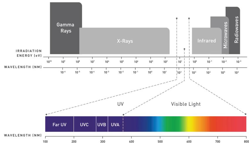
The UV spectrum as shown above is separated into four parts: UVA (315 nm to 400 nm), UVB (280 nm to 315 nm), UVC (200 nm to 280 nm) and UV Vacuum (100 nm to 200 nm)<sup>iii</sup>. Decreasing wavelengths correspond with higher frequency radiation and a higher amount of energy per photon.
